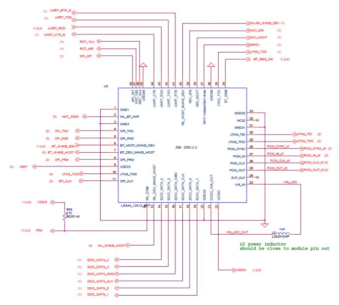
\* PDn need to pull-up to 1.8V/3.3V by 51K resistor
